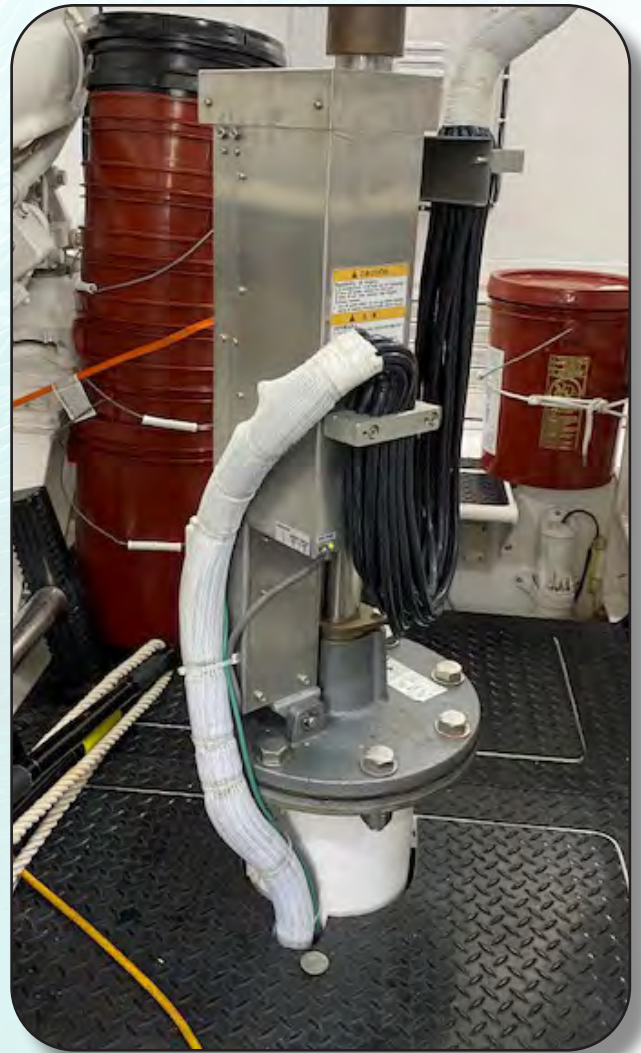
CSH8LMK2 Omni Sonar hull unit installation Photo courtesy of Atlantic Marine Electronics
