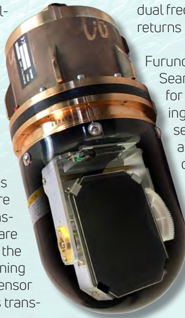
The cutaway shows the inside of a typical Searchlight Sonar dome. The transducer within can be rotated and trained to detect fish and structure at any angle beneath the waterline.
