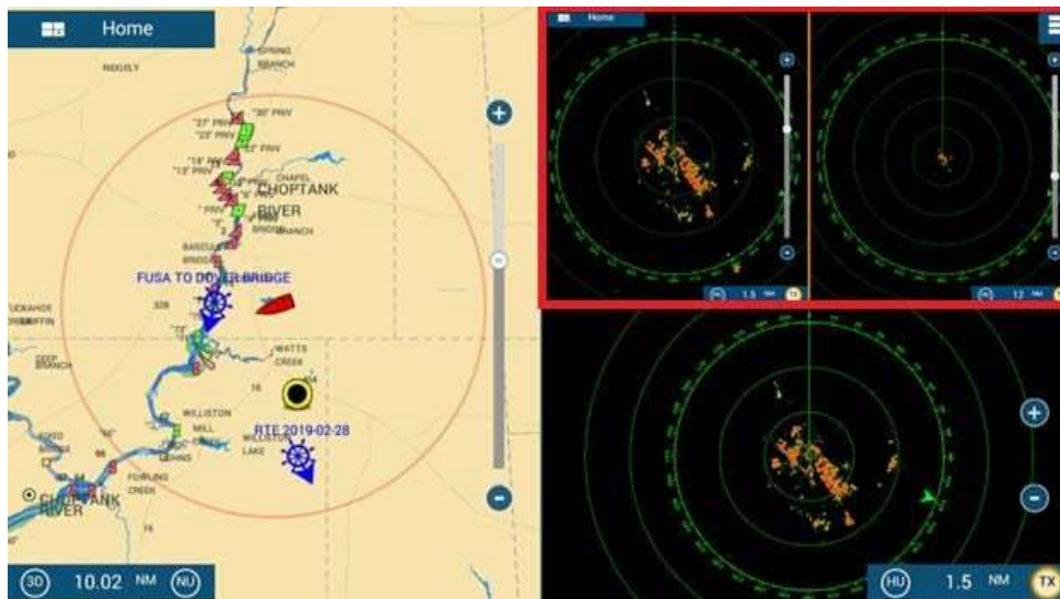
Dual range with one Radar and single range of second Radar on same display
