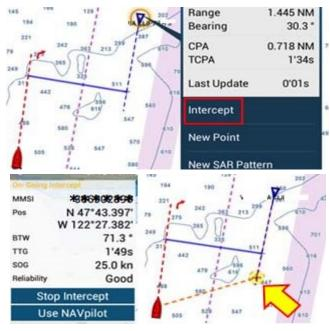
To see details of the meeting point, the Intercept box on the Navigation data box is very efficient, where you can see the details such as the position of selected target.
