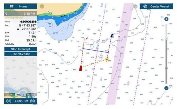
This unique feature can be utilized to find a spot to meet a vessel. As an example, when finding a specific vessel among AIS and ARPA targets on the screen, this feature helps to find the closest spot to meet the
