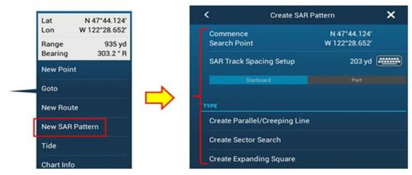
(3) The selected SAR Pattern will appear on the screen. The location, size, and orientation of created SAR
