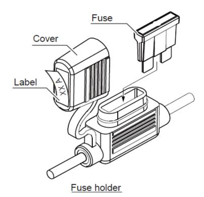
Attach the appropriate supplied label on the fuse holder cover.
