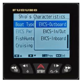
Set [Boat Type] to appropriate EVCS selection. Outboard, In/Out, or Inboard.
