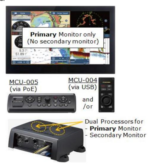
The TZT2BB has dual (2) CPUs for primary and secondary monitors to be controlled independently. In this example, only the Primary monitor is connected to the processor unit. The MCU-005 and/or MCU-004 is used to control the Primary monitor.
