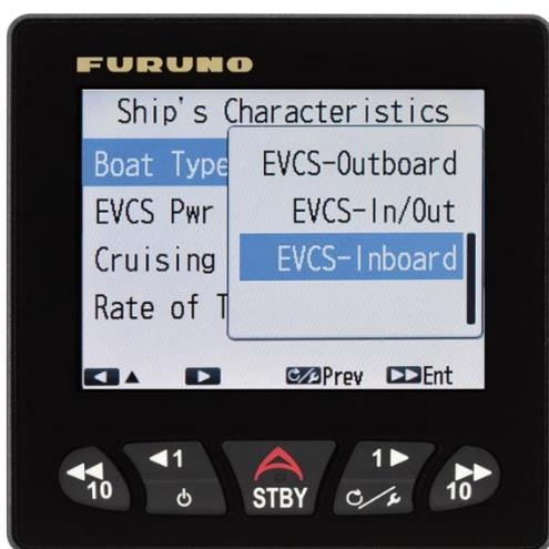
Set [Boat Type] to appropriate EVCS selection. Outboard, In/Out, or Inboard
