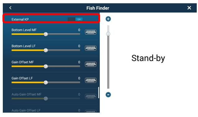
\*Note: Set External KP setting to ON only for the internal/DI fish finder under fish finder menu. **DO NOT** set External KP to ON within the Multi-Beam Sonar menu. Not following this will cause the Multi-beam to stop transmitting.
