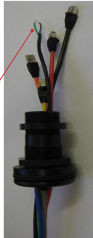
Figure 12. Gland Assembly - Cable Connectors
