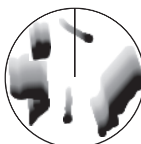
Relative echo trails (Targets moving relative to own ship)
