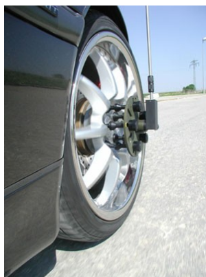
Illustration 25: Aftermarket wheel speed sensor
