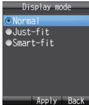
2. Pulse **▲** o **▼** para seleccionar [Normal], [Just-fit] o [Smart-fit].
