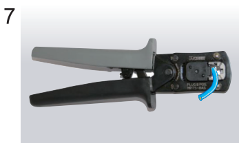
7 Using special crimping tool MPT5-8AS (PANDUIT CORP.), crimp the modular plug. Finally, check the plug visually.
