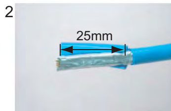
Remove the outer sheath by approx 25 mm. Be careful not to damage inner shield and cores.
