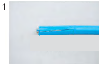
Expose inner vinyl sheath.
