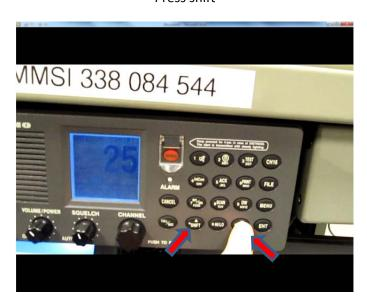
Then while shift is active, (shown in upper right of LCD) press down arrow and up arrow to increase and decrease contrast.
