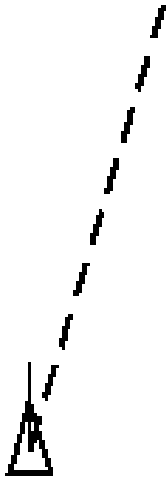
AIS dangerous target blinking red until acknowledged, then it is displayed as red symbol.
