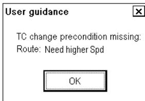
**Reason:** Change of route steering mode when speed of vessel is less than defined for route steering.
