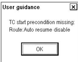
**Reason:** If alert 471 has been generated and later condition for alert 471 disappears without changing steering mode from NAVI to AUTO or HAND.
