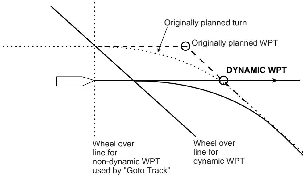
*How the location of a Dynamic WPT is defined when the NAVI steering mode is in use*
