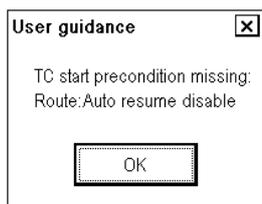
**Reason:** If alert 471 has been generated and later the condition for alert 471 is resolved without changing steering mode from NAVI to AUTO or HAND.
