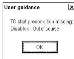
**Reason:** You tried to activate a route steering mode when there is a difference between current heading and the required set heading that is greater than set with **Route start limit angle** in the Route Parameters dialog box.
