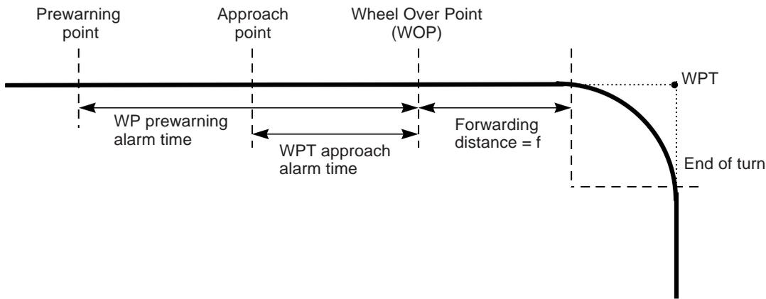
As soon as your ship arrives to a wheel over point, the ECDIS sends a new course command to the autopilot and the maneuver is started. During a maneuver, the radar display and the ECDIS display show the curved EBL, indicating the planned radius for maneuver.
