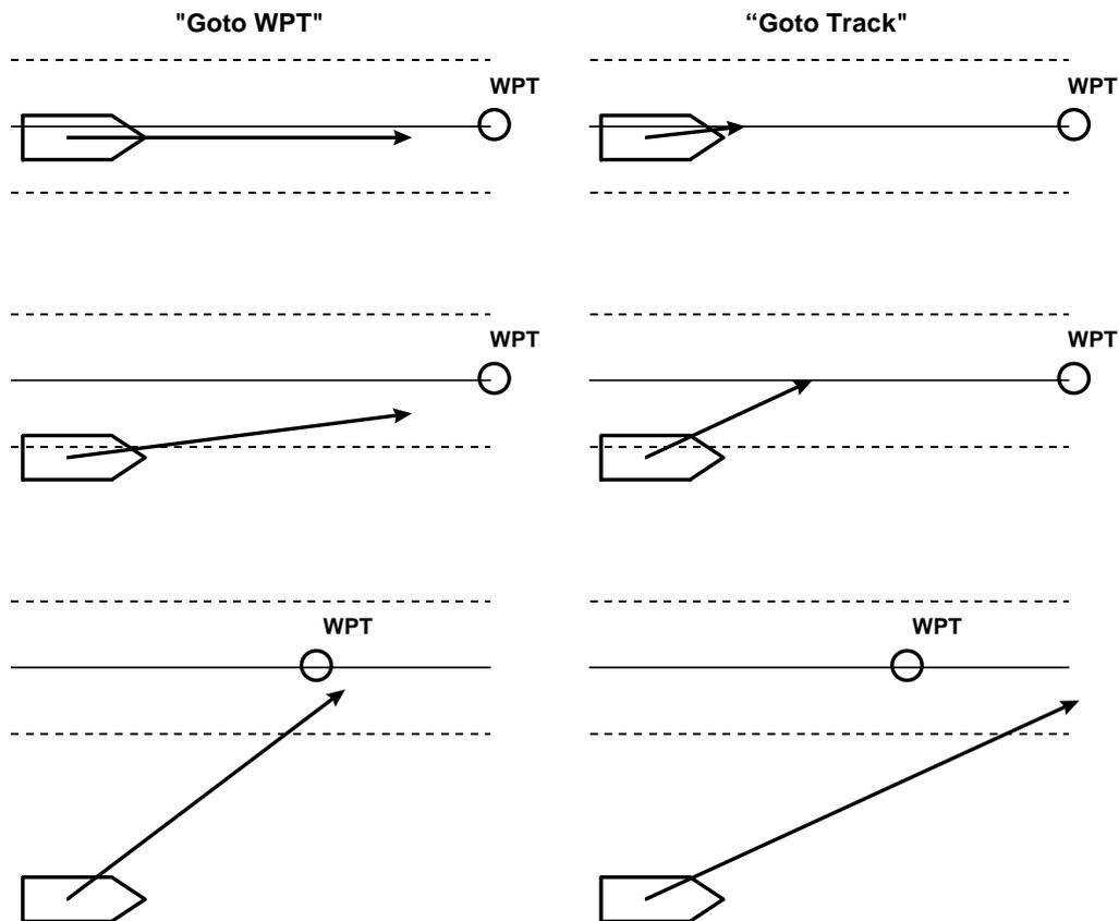
**Note:** If the off track error is more than 100 meters in the Goto Track mode, the system cannot increase the approach angle towards the center line of the route.
