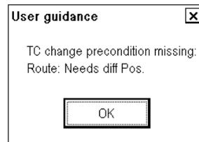
**Reason:** Change steering mode from GoAW to GoSEA without high precision positioning device (GPS in differential correction mode).
