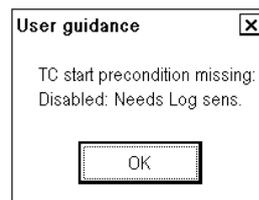
**Reason:** You tried to activate a route steering mode without an independent speed source. You need either a log, a dual-axis log or two position receivers.
