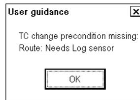
**Reason:** Change of route steering mode without independent speed source. You need either a log, a dual-axis log or two position receivers.
