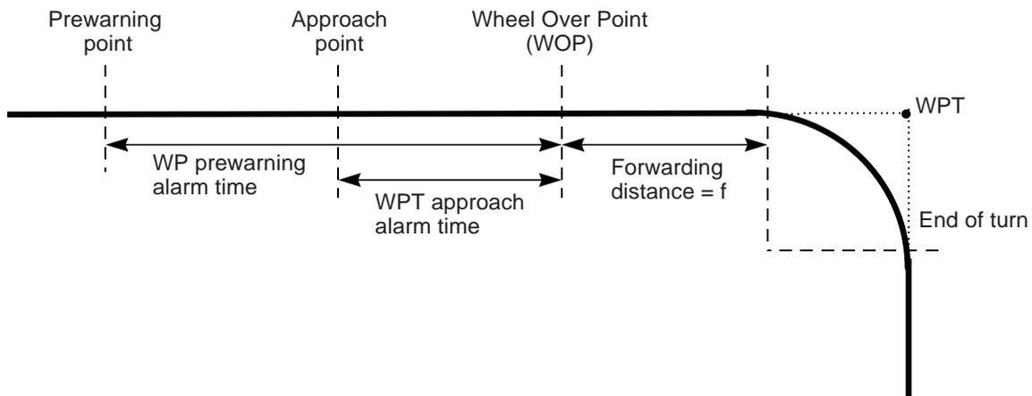
As soon as the ship arrives at the wheel over point, the ECDIS sends a new course command to the autopilot and the maneuver is started. During a maneuver, the radar display and the ECDIS display show the curved EBL that shows the planned radius for a maneuver.
