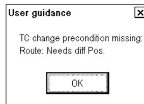
**Reason:** Changed steering mode from GoSEA to GoAW steering without high precision positioning device (GPS in differential correction mode).
