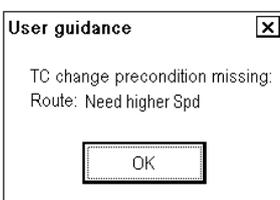
**Reason:** Change of route steering mode when speed of ship is less than defined for route steering.
