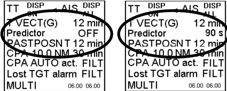
The predictor is calculated using current speed and rate of turn:
