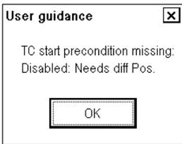
**Reason:** You tried to activate the GoAW steering mode without a high-precision positioning device (GPS in differential correction mode).
