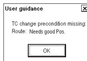
**Reason:** Change of route steering mode when Alert "407 Position discrepancy" is active.
