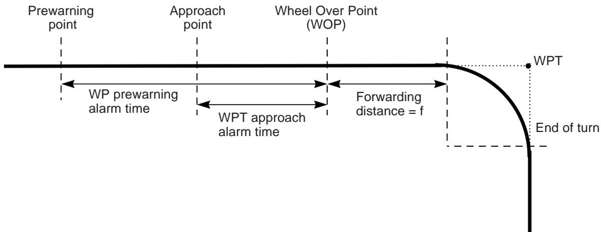
As soon as the ship arrives at the wheel over point, the ECDIS sends a new course command to the autopilot FAP-2000 and the corresponding maneuver is initiated. During a maneuver, both the radar display and the ECDIS display show the curved EBL, indicating the planned radius for the maneuver.
