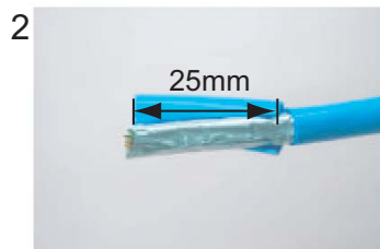
Remove the outer sheath by approx 25 mm. Be careful not to damage inner shield and cores.
