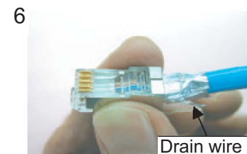
Insert the cable into the modular plug so that the folded part of the shield enters into the plug housing. The drain wire should be located on the tab side of the jack.
