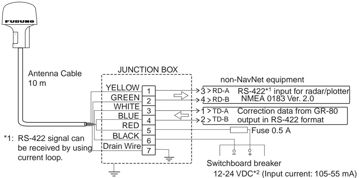
**Note 1:** When connecting FURUNO DGPS beacon receiver GR-80 to this unit, set it as follows:
