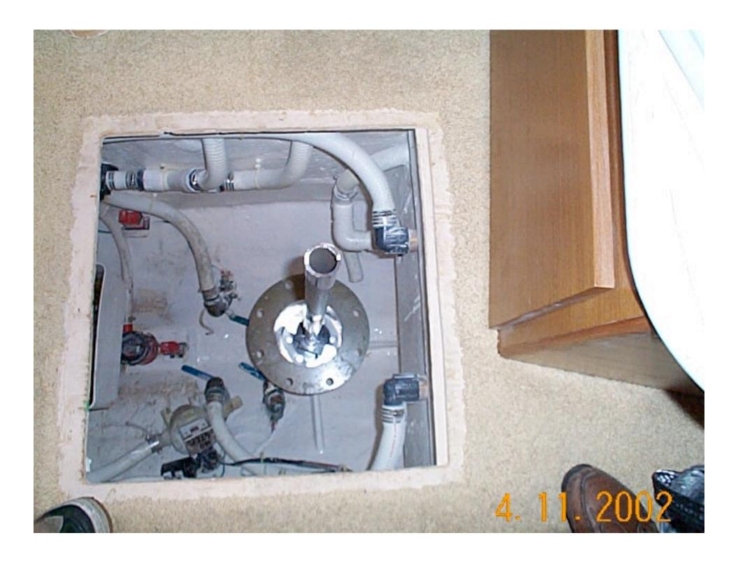
You can see why we need the SS shims and the installer needs to hand fit by filing the guides by hand. At first fit the contact point is to small. See the black smear.
